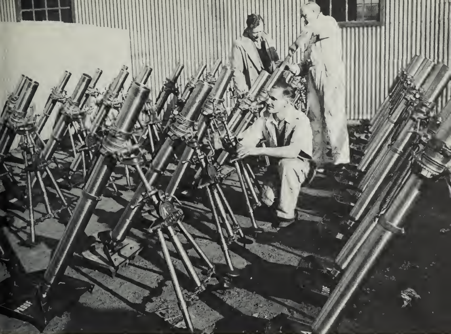
Assembling a batch of South African-made mortars. Much of the plant for turning out urgently needed Army requirements was improvised on the spot.
